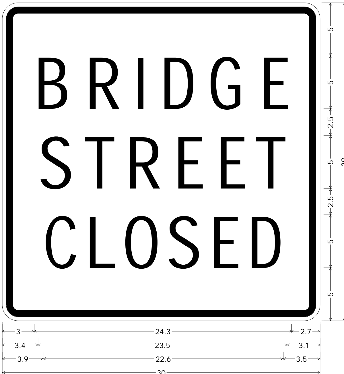
R4-1 STD; 1.5" Radius, 0.6" Border, 0.4" Indent, Black on White; "BRIDGE" D 125% spacing; "STREET" D; "CLOSED" D 60% spacing;
